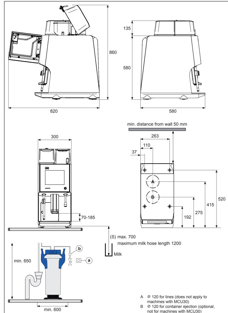
The Melitta® Cafina® XT6 is delivered ready for connection. However, before setting it up, the connections required on site must have been installed so that they are easily accessible within a radius of 1 m. This preliminary work must be carried out by authorized specialists in compliance with the applicable regulations. Melitta® Customer Services is not authorized to carry out this work and does not assume any responsibility for the installation.
